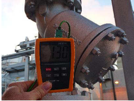
Uninsulated – primed pipework- 130°C (266°F)
